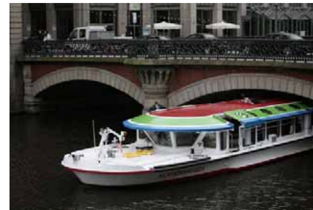
Retractable roof to pass under bridges
